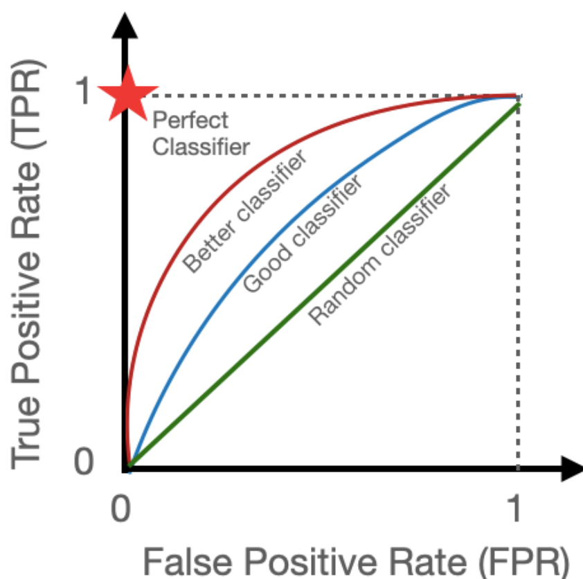
Σχήμα 3.8: Καμπύλη ROC (Receiver Operating Characteristic) όπου TPR = RECALL
