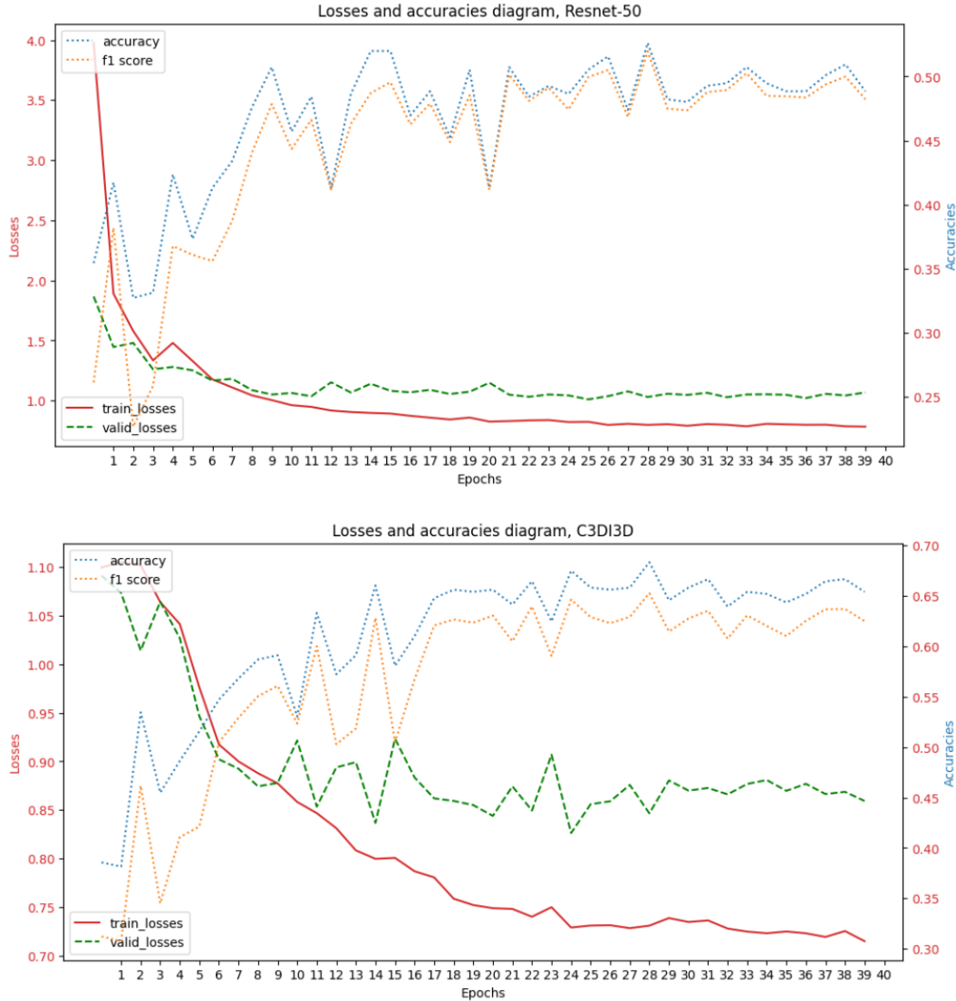
Figure 4.4.6: Comparison of the losses, accuracy and F1 score of the two different models during training.
