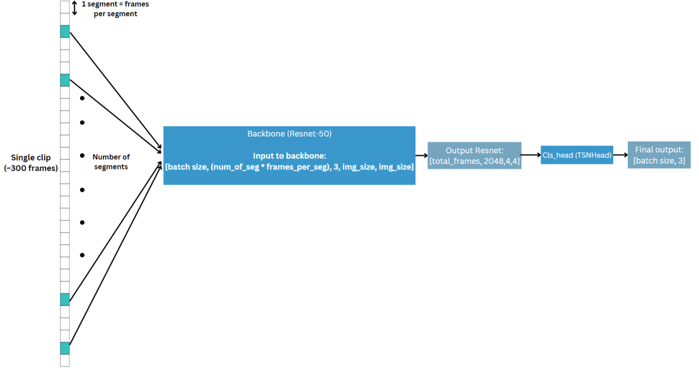
Figure 4.4.1: ResNet-50-TSN architecture used for the engagement estimation problem on the Pinsoro dataset [44].
