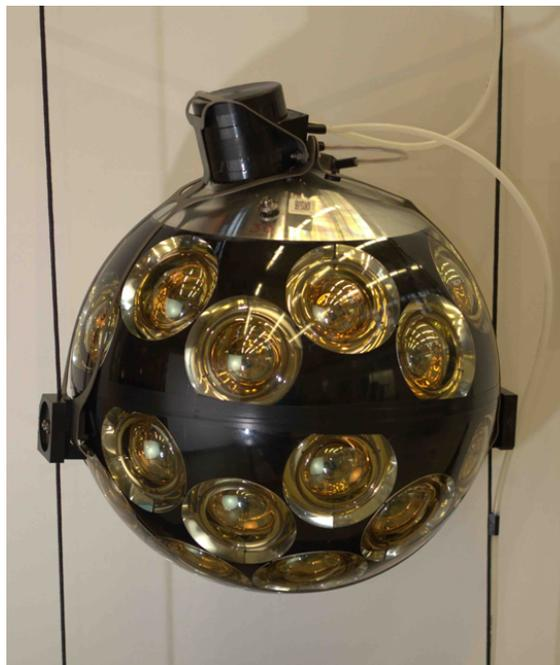
Figure 3.2: A KM3NeT multi-PMT Digital Optical Module (DOM). From [28].
