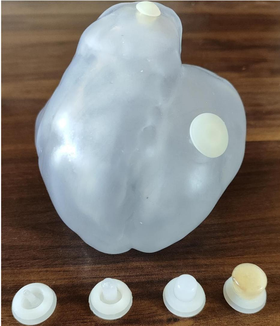
**Figure 4.18: Final 3D printed cardiac phantom with 4 silicone plugs-blockages**
