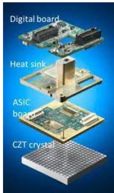
Figure 2.9: CZT module basic components (8)
