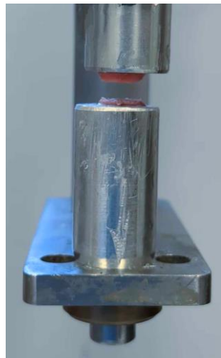
Figure 8: A representative photograph of the end stage of a successful direct tension test.
