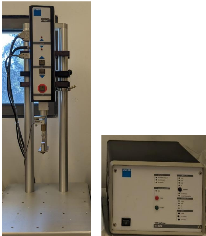
Figure 7: Experimental setup, the tensile machine consists of the main tensile unit and the control unit.
