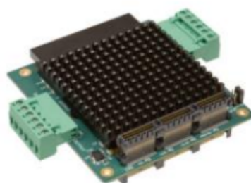
(shown with pin fin heat sink installed)
