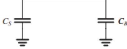
Figure 3.3: When the voltage of the selected word line is raised, the transistor conducts, thus connecting the storage capacitor with the bitline capacitor.
