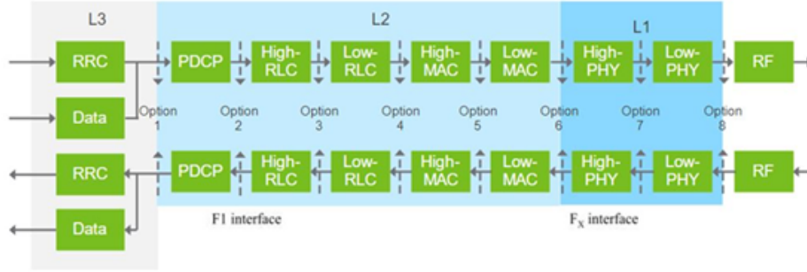
Figure 3.1: Signal processing functions in the protocol stack and different Functional Split options provided by 3GPP [5].
