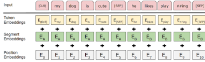
Figure 3.2: BERT input representation. The input embeddings are the sum of the token embeddings, the segmentation embeddings and the position embeddings. Source: [14]
