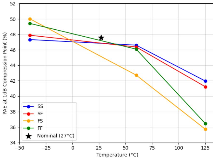
Figure 8.6: PAE at 1 dB compression point across process and temperature corners for the two-stage power amplifier
