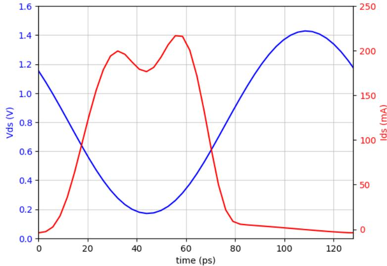
Figure 5.15: Voltage and current waveforms at the 1 dB compression point in Class B operation
