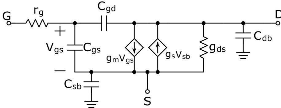
Figure 4.3: Equivalent high-frequency model of the MOS transistor
