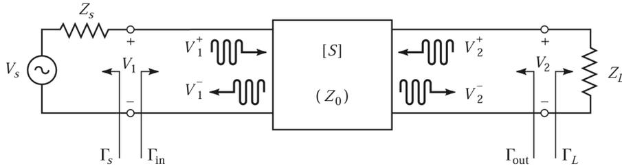
Figure 4.2: Two-port network with an AC voltage source  $V_s$  at the input, a source resistance  $Z_s$ , and a load resistance  $Z_L$  at the output [2]
