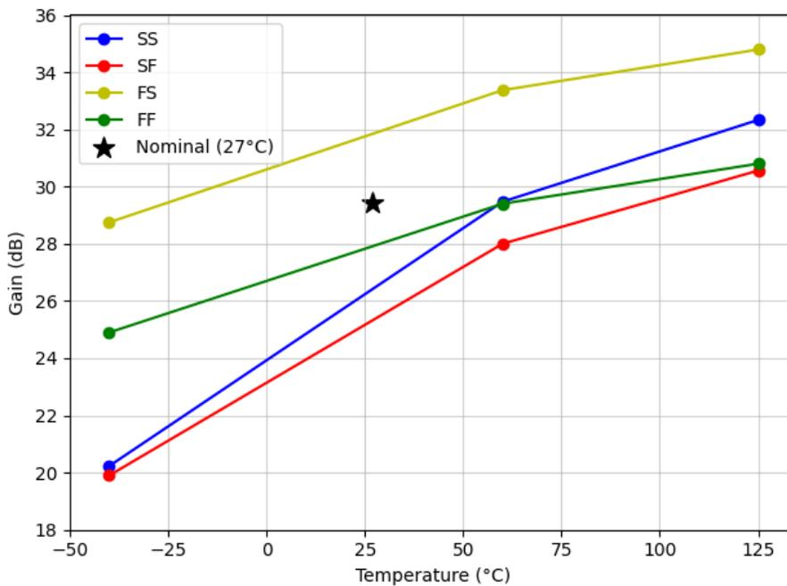
Figure 8.4: Gain performance across process and temperature corners for the two-stage power amplifier
