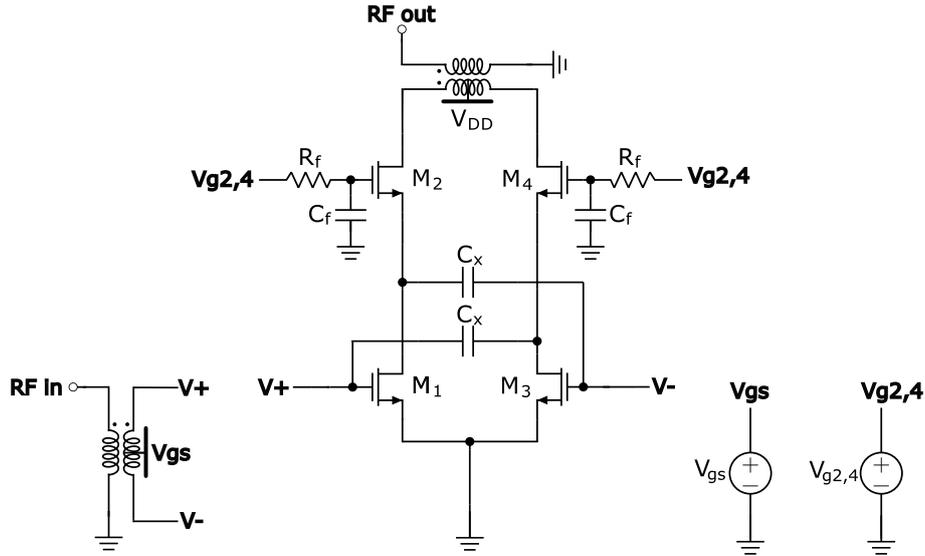
Figure 5.24: Cascode differential power amplifier
