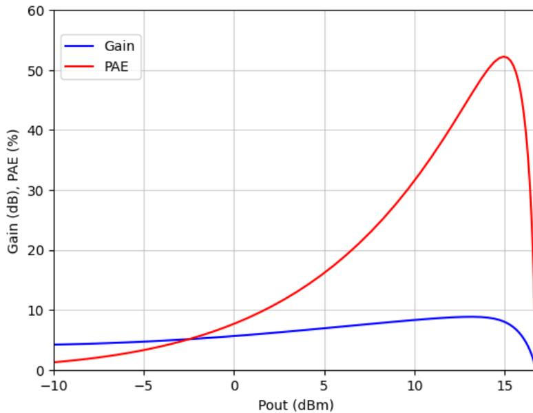
Figure 5.16: Gain and PAE versus output power for Class C operation
