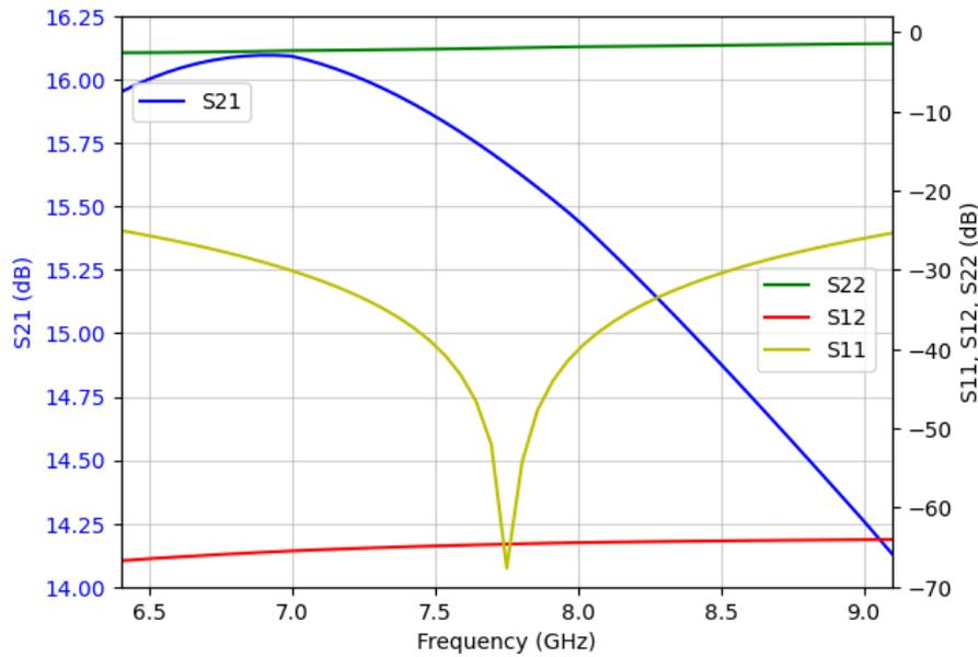
Figure 6.24: Post-layout  $S$ -parameters of the power amplifier stage
