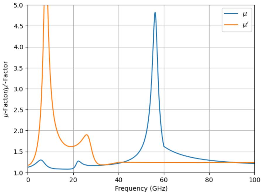
Figure 8.2: Stability factors  $\mu$  and  $\mu'$  of the two-stage power amplifier
