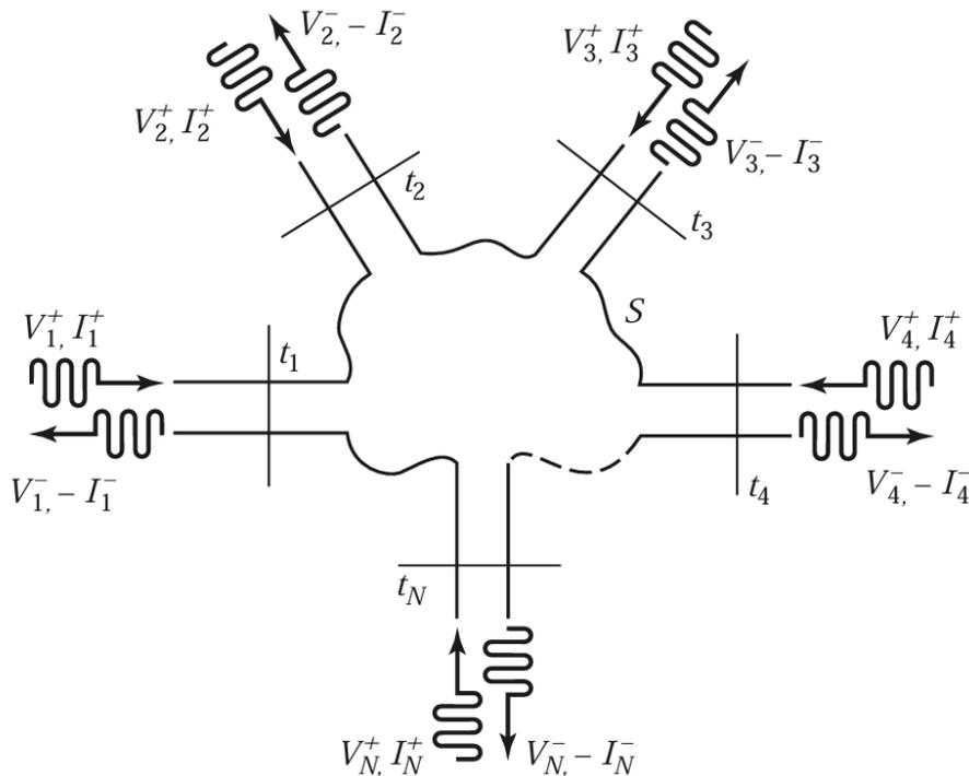
Figure 4.1: N-port microwave network [2]
