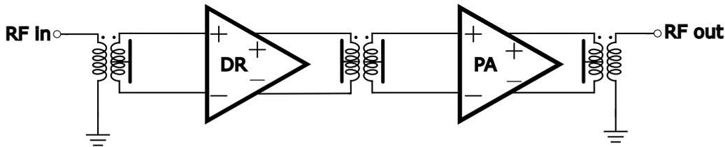
Figure 5.26: Two-Stage Power Amplifier
