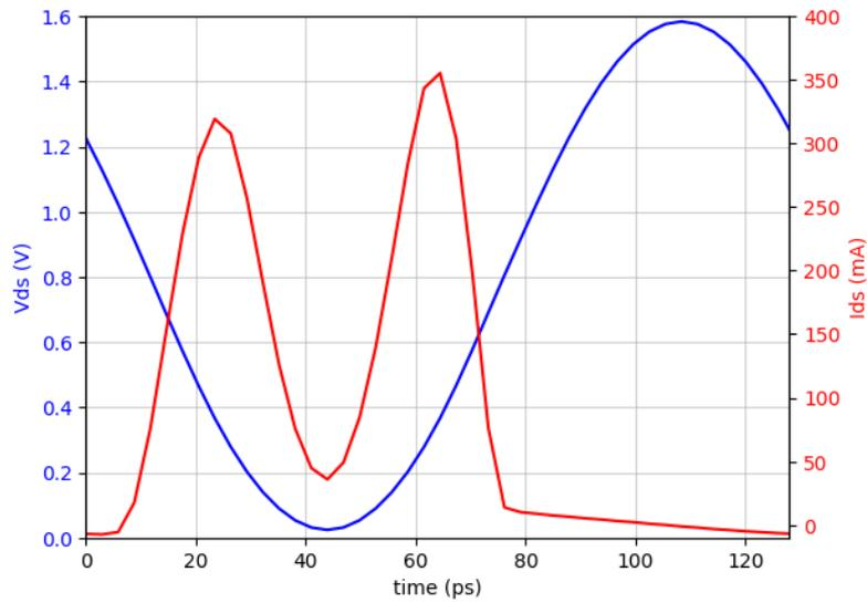
Figure 5.17: Voltage and current waveforms at the 1 dB compression point in Class C operation
