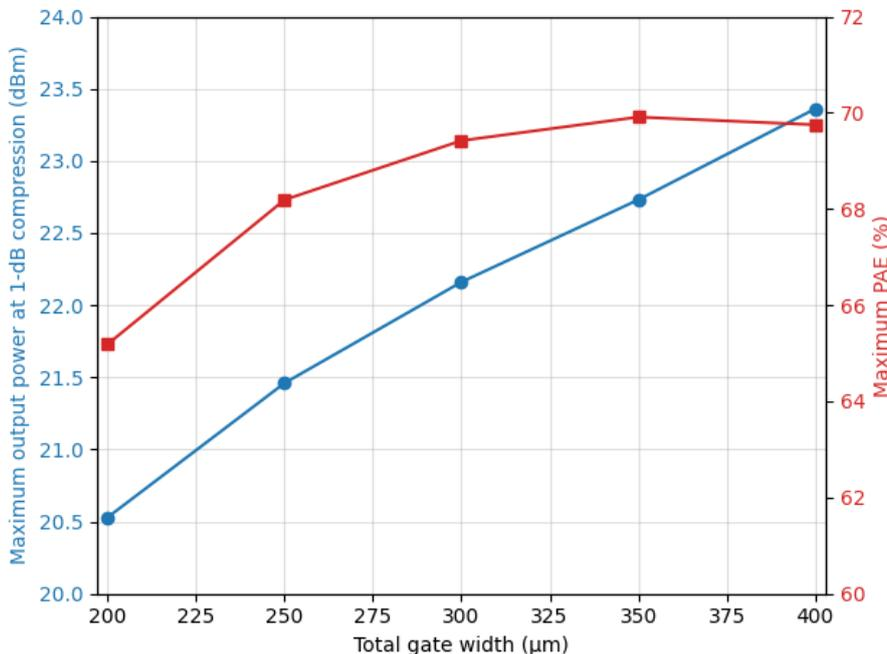
Figure 6.2: Maximum output power at 1 dB compression point and maximum PAE versus total gate width
