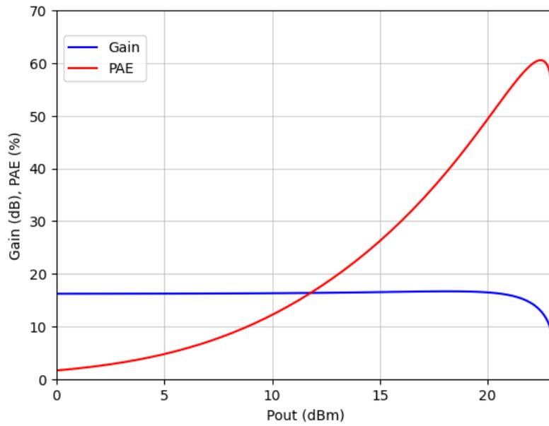
Figure 5.25: Gain and PAE versus output power for the cascode differential power amplifier in Class B operation
