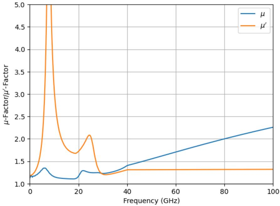
Figure 8.9: Post-layout stability factors  $\mu$  and  $\mu'$  of the two-stage power amplifier
