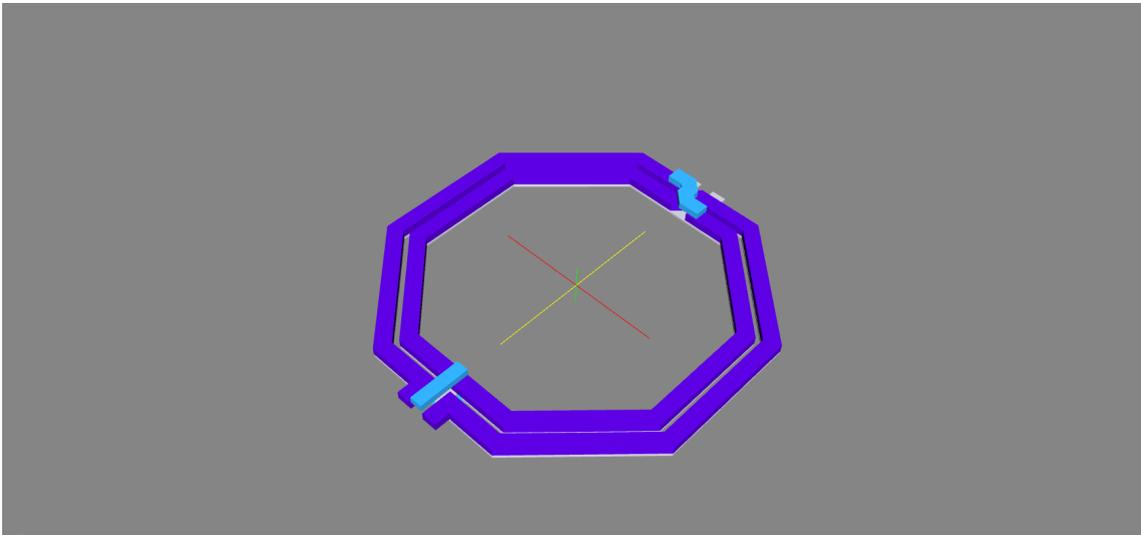
Figure 7.6: Stacked input balun layout
