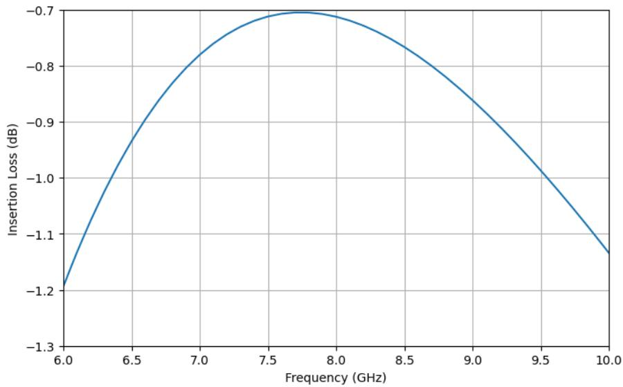
Figure 7.5: Insertion loss of the interstage transformer including the matching capacitor  $C_{m2}$
