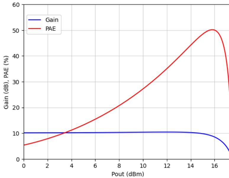
Figure 5.14: Gain and PAE versus output power for Class B operation
