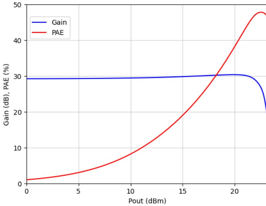
Figure 8.1: Gain and PAE versus output power of the two-stage power amplifier
