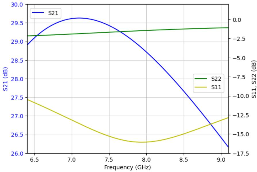
Figure 8.3: S-parameters of the two-stage power amplifier
