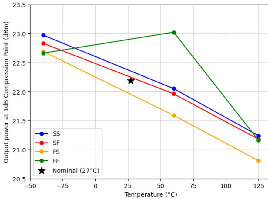
Figure 8.5: Output power at 1 dB compression point across process and temperature corners for the two-stage power amplifier
