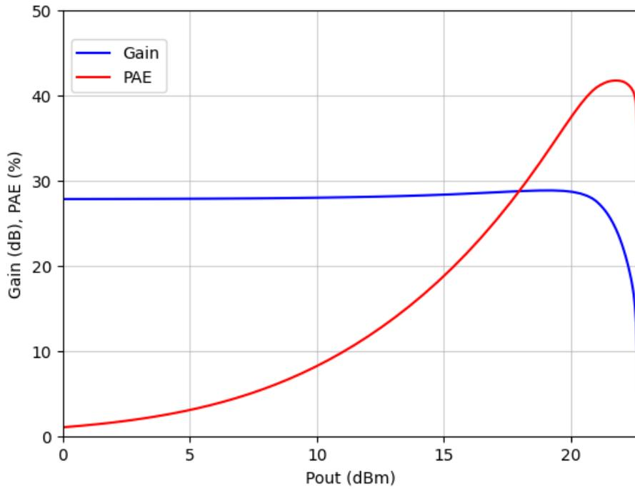
Figure 8.8: Post-layout gain and PAE versus output power of the two-stage power amplifier
