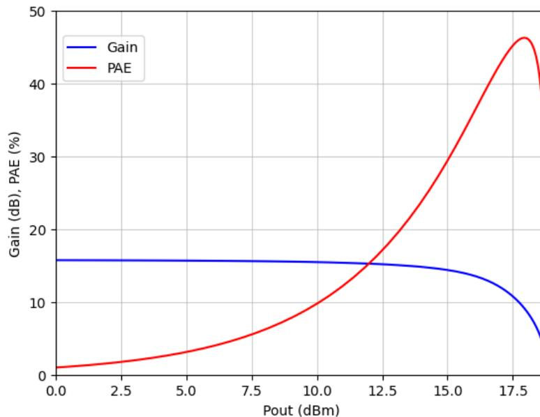
Figure 5.10: Gain and PAE versus output power for Class A operation
