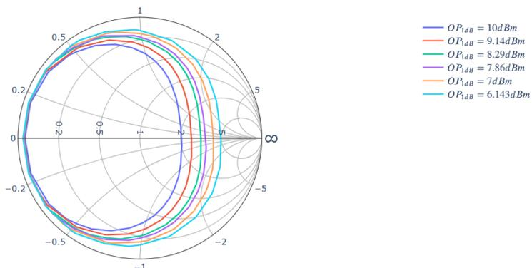
Figure 7.2: 1 dB compression point contours
