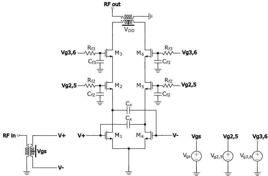
Figure 5.22: Three-stacked power amplifier
