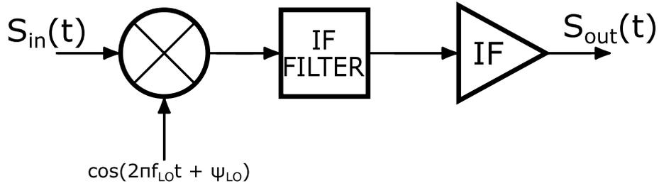
Figure 2.4: Intermediate Frequency stage
