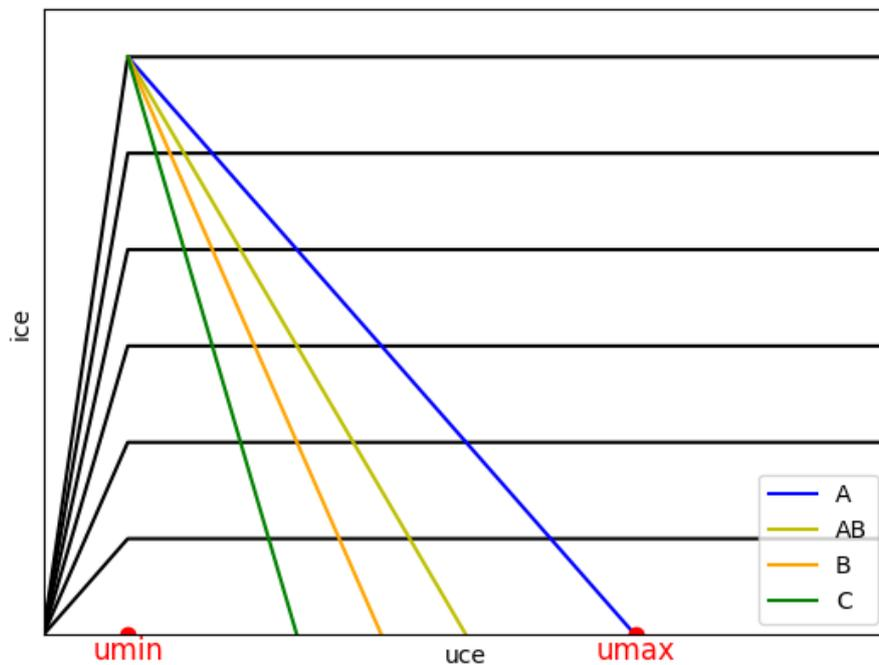
Figure 5.8: IV curves with corresponding load lines for different amplifier classes
