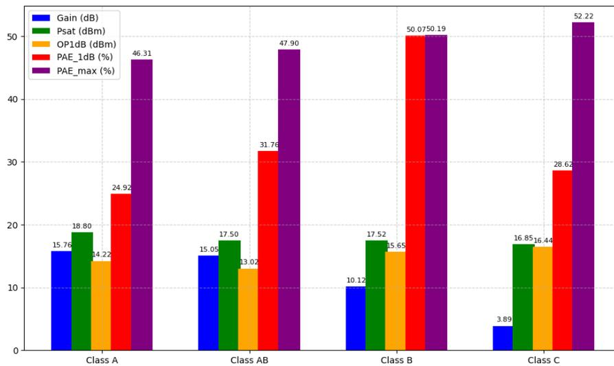
Figure 5.18: Performance Comparison Across Basic Power Amplifier Classes
