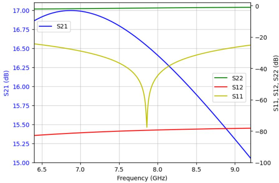
Figure 6.15: S-parameters of the power amplifier stage
