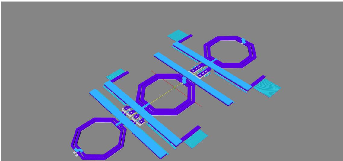
Figure 8.7: Layout of the complete two-stage power amplifier
