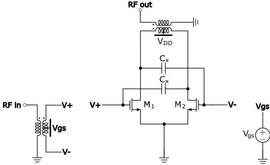
Figure 5.19: Differential common-source power amplifier
