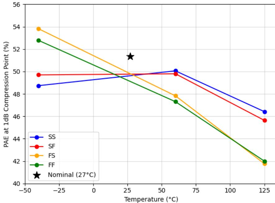
Figure 6.18: PAE at 1dB compression point across process and temperature corners for the power amplifier stage
