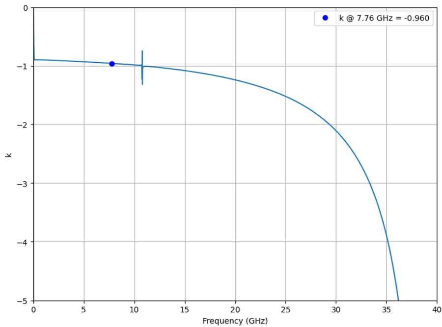
Figure A.5: Coupling Factor ( $k$ ) versus frequency for the output balun
