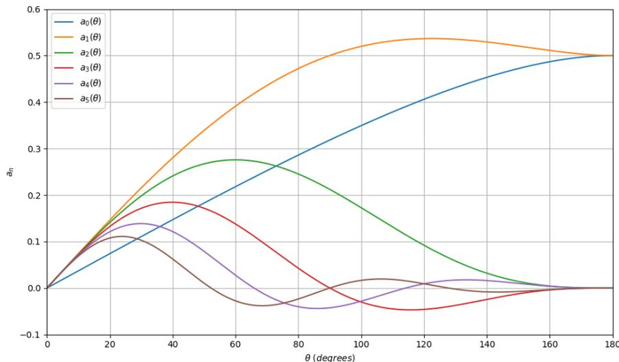
Figure 5.3: Plots of the harmonic amplitude coefficients  $a_n(\theta)$  for the DC, the fundamental, and higher-order harmonic components
