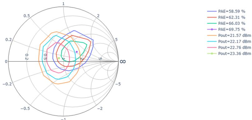
Figure 6.5: Load-pull simulation at the optimal input-referred 1 dB compression point
