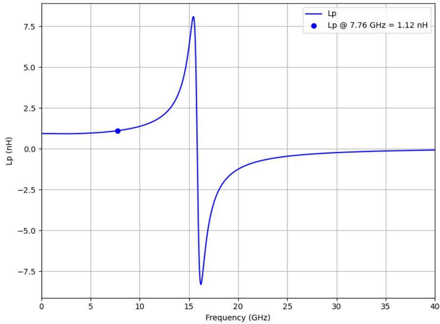
Figure A.6: Primary Inductance ( $L_p$ ) versus frequency for the input balun
