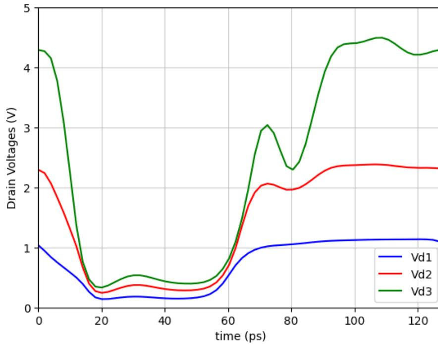
Figure 6.10: Drain voltages with the RC network included
