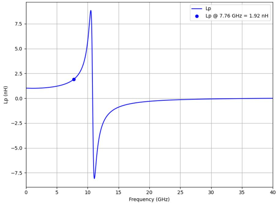
Figure A.2: Primary Inductance ( $L_p$ ) versus frequency for the output balun
