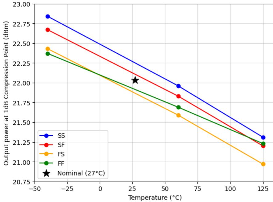
Figure 6.17: Output power at 1dB compression point across process and temperature corners for the power amplifier stage
