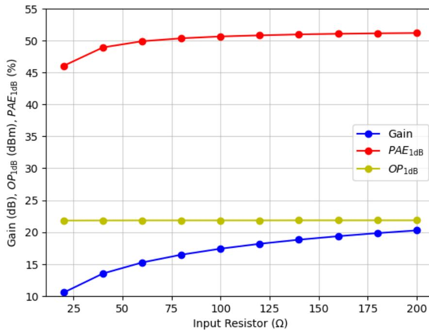
Figure 6.11: Performance metrics versus input resistor value
