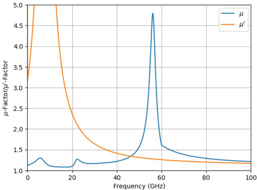
Figure 6.14: Stability factors  $\mu$  and  $\mu'$  of the power amplifier stage
