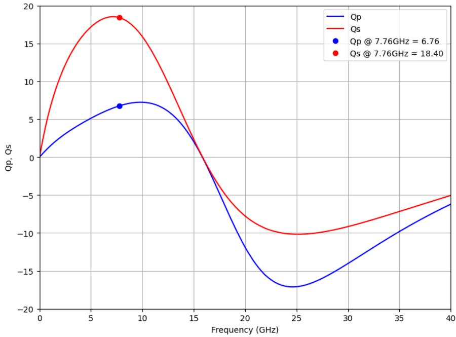
Figure A.8: Quality Factors ( $Q_p$ ,  $Q_s$ ) versus frequency for the input balun
