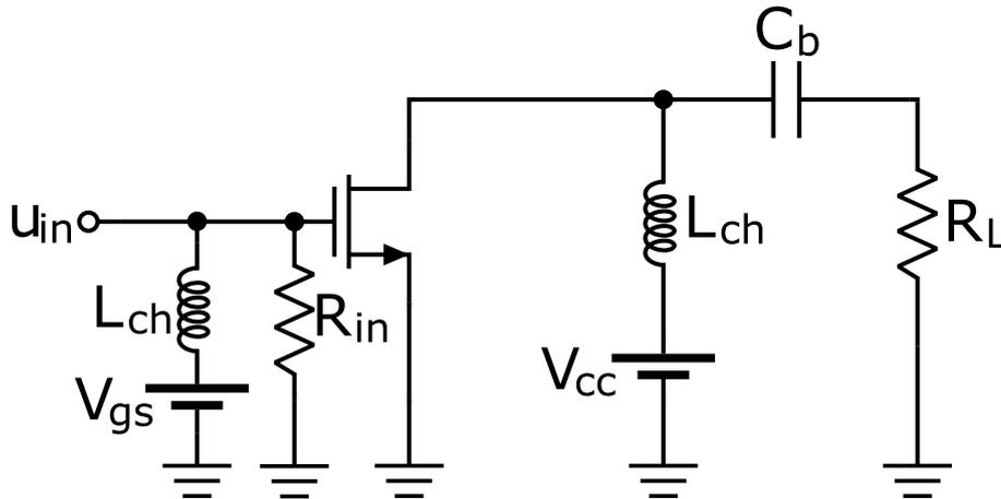
Figure 5.9: Common-source power amplifier
