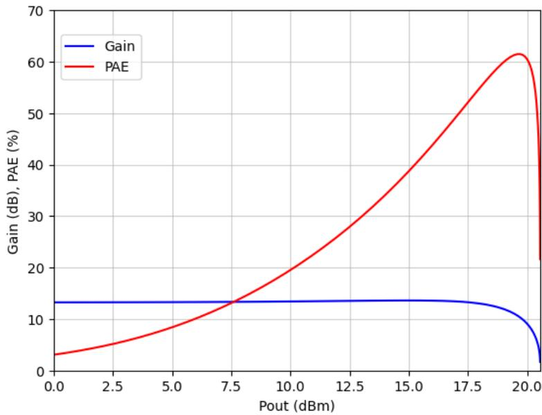
Figure 5.21: Gain and PAE versus output power for the Differential Power Amplifier in Class B operation
