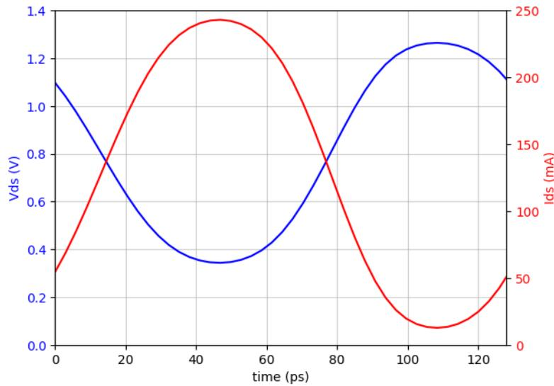
Figure 5.11: Voltage and current waveforms at the 1 dB compression point in Class A operation
