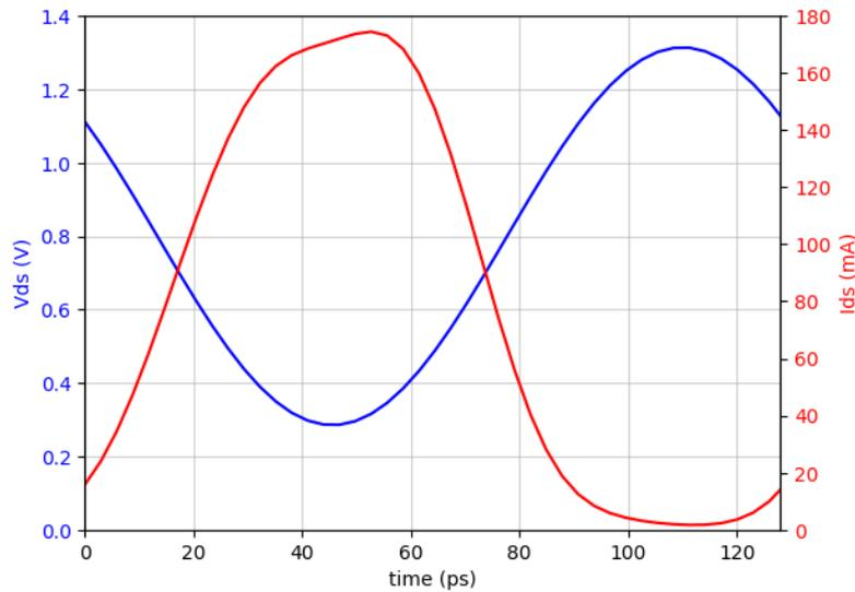
Figure 5.13: Voltage and current waveforms at the 1 dB compression point in Class AB operation
