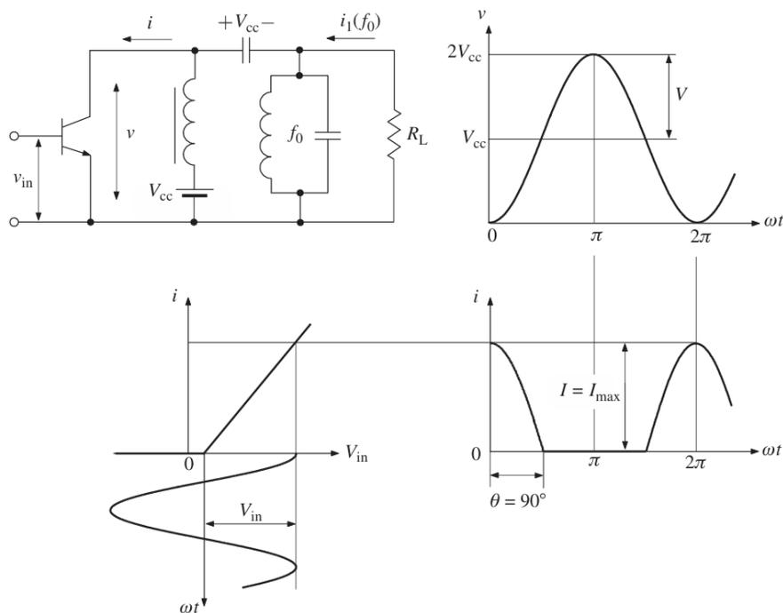
Figure 5.5: Voltage and current waveforms in Class B operation [3]
