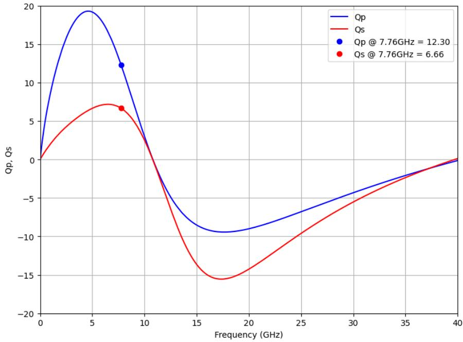
Figure A.4: Quality Factors ( $Q_p$ ,  $Q_s$ ) versus frequency for the output balun
