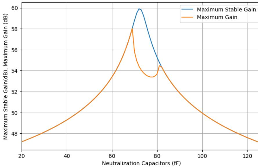
Figure 6.4: Maximum gain and maximum stable gain versus  $C_x$ .
