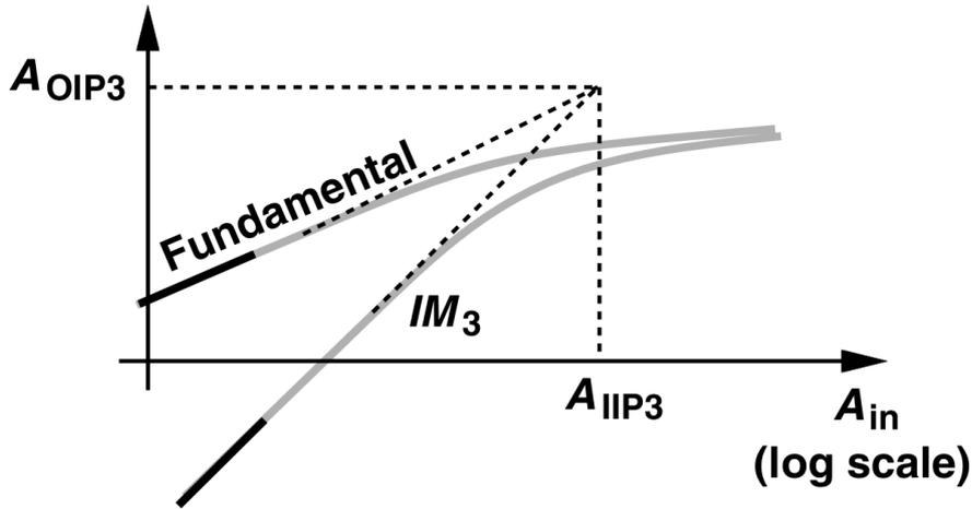
Figure 3.3: Definition of IP3 based on extrapolation [1]
