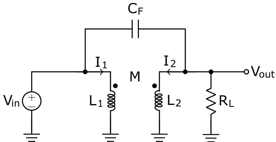
Figure A.1: Simplified transformer equivalent circuit
