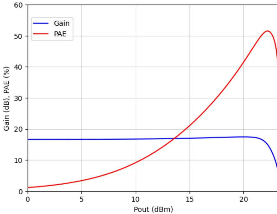
Figure 6.13: Gain and PAE versus output power of the power amplifier stage
