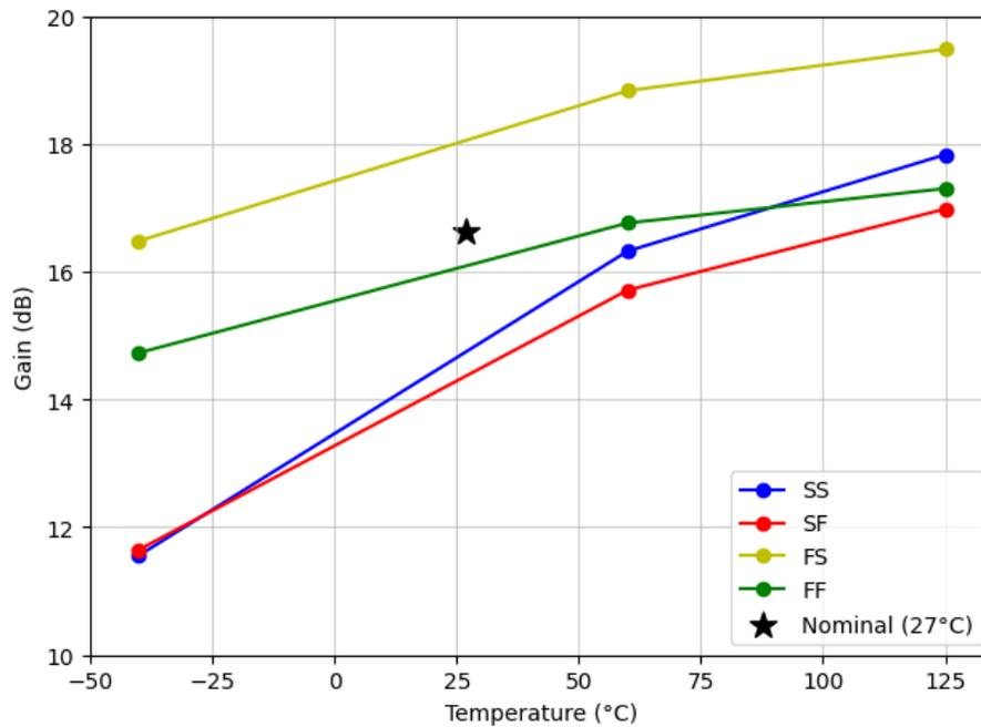
Figure 6.16: Gain performance across process and temperature corners for the power amplifier stage
