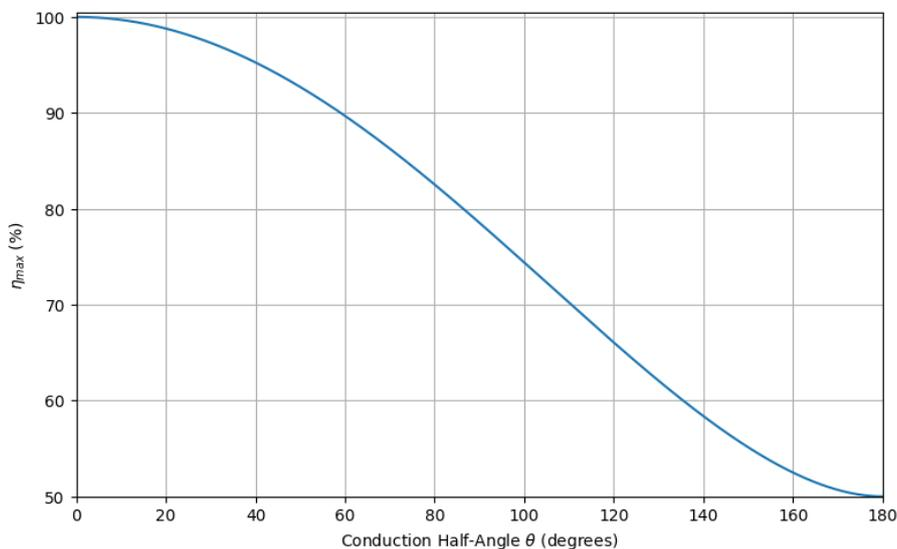
Figure 5.6: Maximum theoretical efficiency as a function of the conduction half-angle  $\theta$
