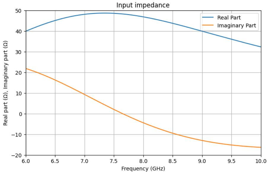
Figure 6.7: Input impedance of the output balun including the matching capacitor  $C_m$
