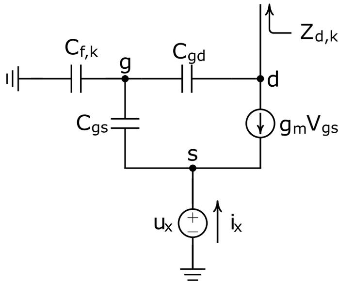
Figure 5.23: Small-signal equivalent circuit of the  $k$ -th transistor
