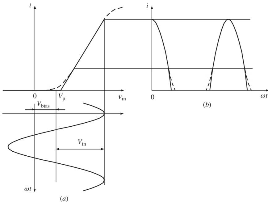
Figure 5.1: Piecewise linear approximation technique [3]
