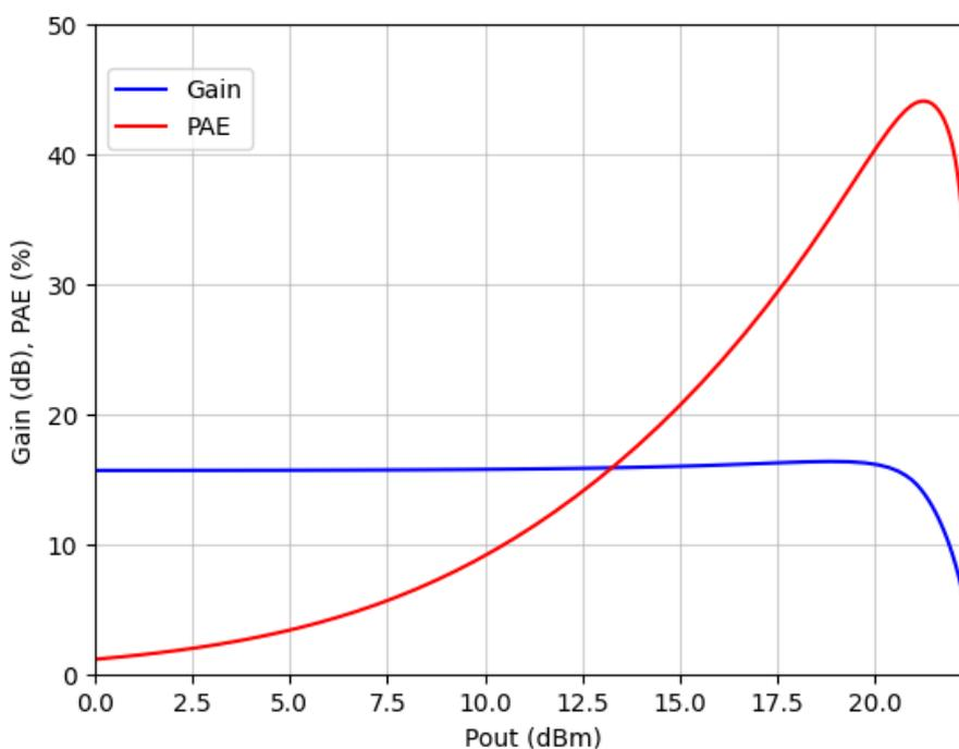
Figure 6.22: Post-layout Gain and PAE versus output power of the power amplifier stage
