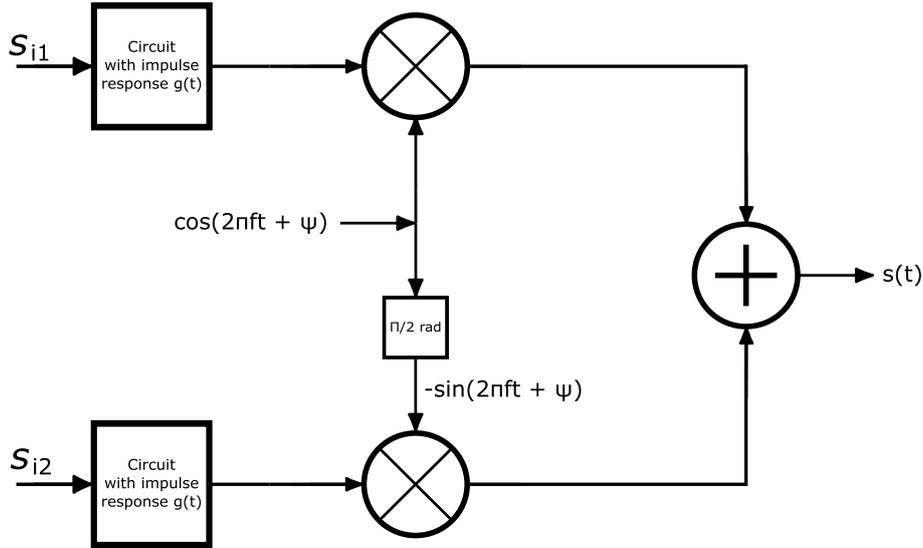
Figure 2.2: The orthogonal modulator along with the pulse shaping circuit
