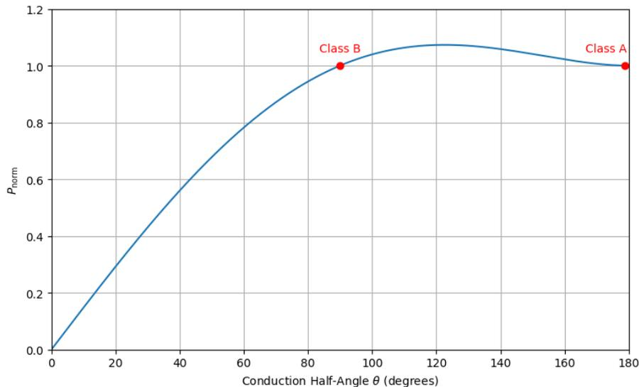
Figure 5.7: Normalized output power  $P_{\text{norm}}$  as a function of the conduction half-angle  $\theta$ .
