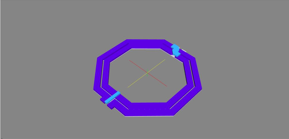
Figure 6.6: Stacked output balun layout
