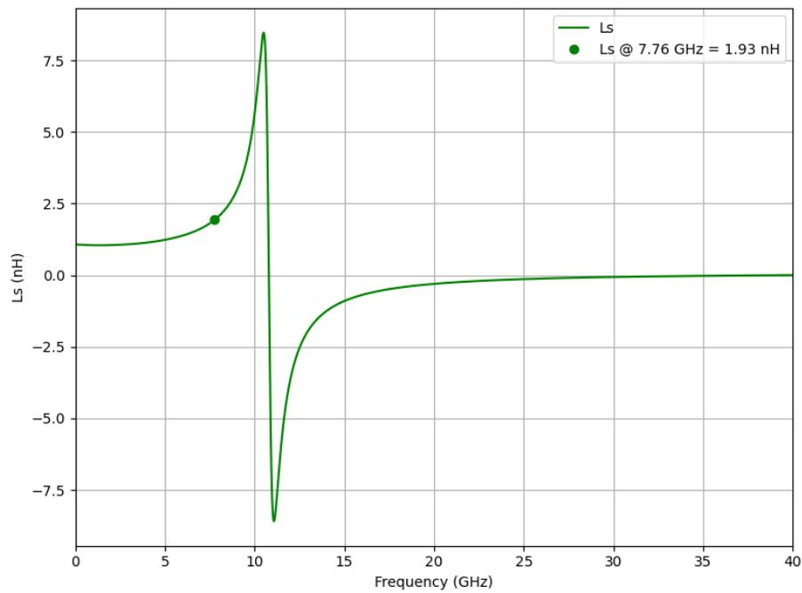
Figure A.3: Secondary Inductance ( $L_s$ ) versus frequency for the output balun
