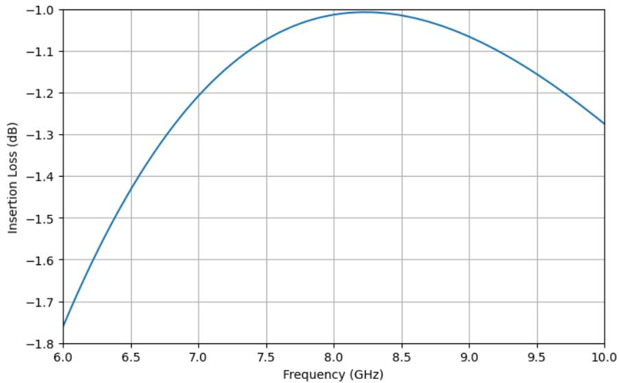
Figure 7.8: Insertion loss of the input balun including the matching capacitor  $C_{m1}$
