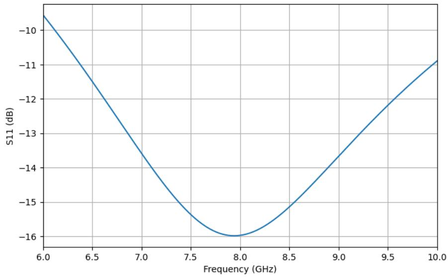
Figure 7.7:  $S_{11}$  parameter of the input balun including the matching capacitor  $C_{m1}$
