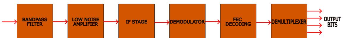
Figure 2.3: Superheterodyne Receiver
