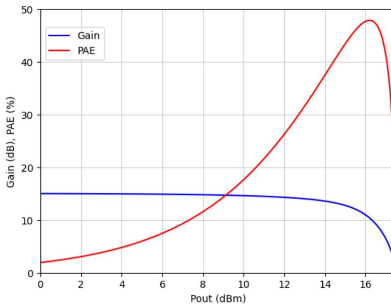
Figure 5.12: Gain and PAE versus output power for Class AB operation
