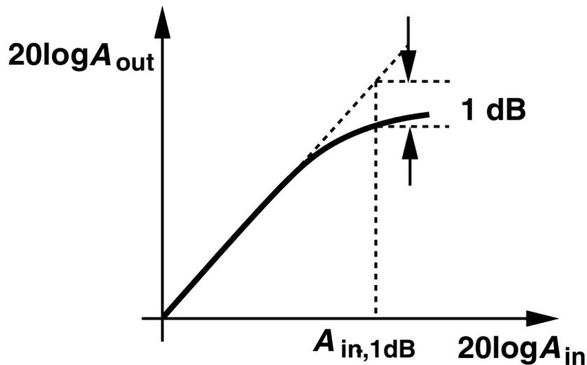
Figure 3.2: Input-output power characteristic of a nonlinear system [1]
