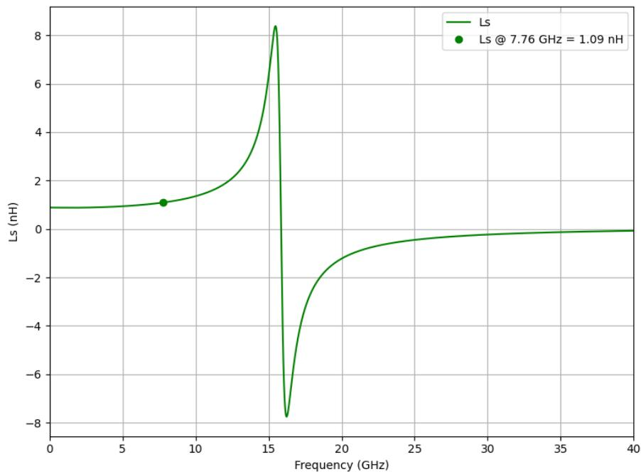
Figure A.7: Secondary Inductance ( $L_s$ ) versus frequency for the input balun
