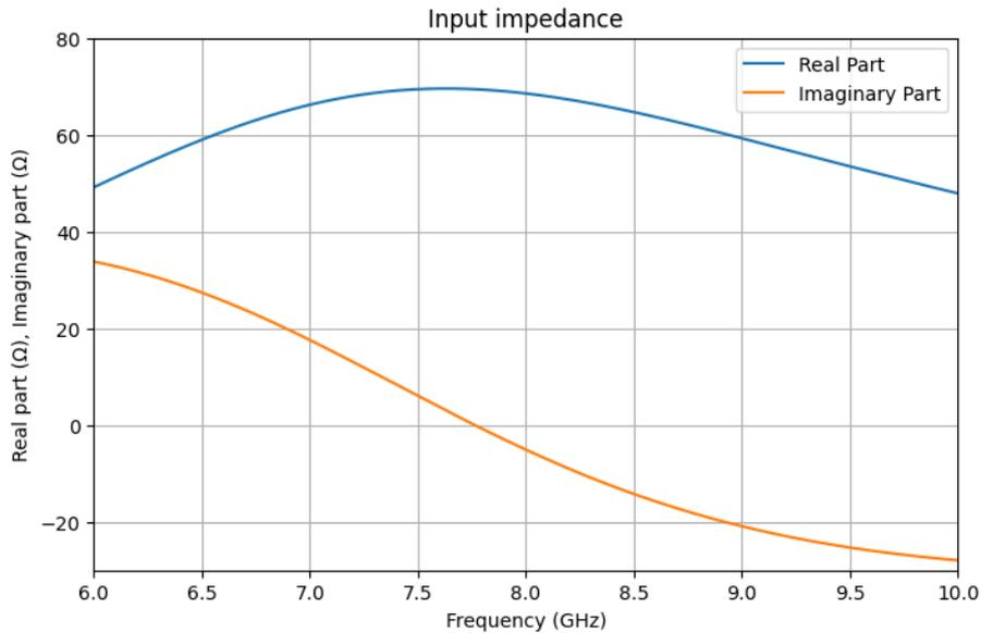
Figure 7.4: Input impedance of the interstage transformer including the matching capacitor  $C_{m2}$
