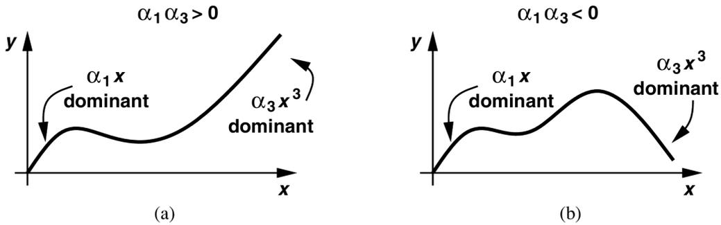
Figure 3.1: (a) Expansive and (b) Compressive characteristics [1]
