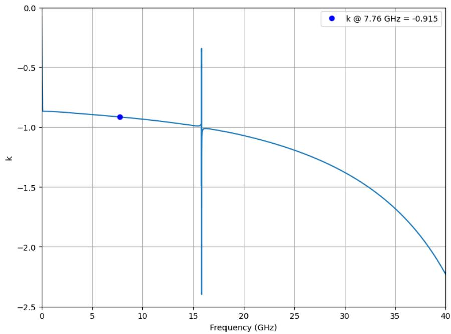
Figure A.9: Coupling Factor ( $k$ ) versus frequency for the input balun
