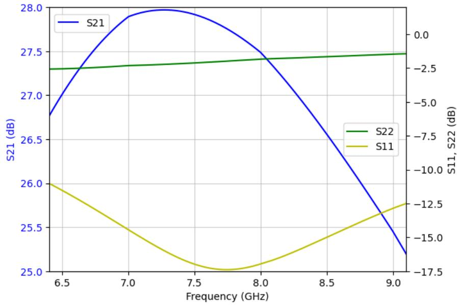
Figure 8.10: Post-layout S-parameters of the two-stage power amplifier
