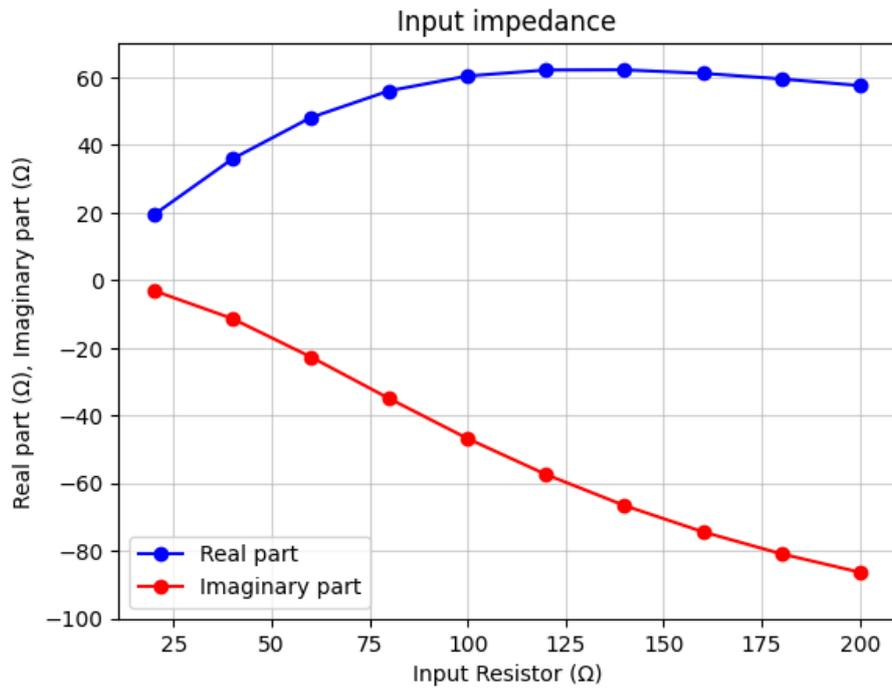
Figure 6.12: Input impedance versus input resistor value
