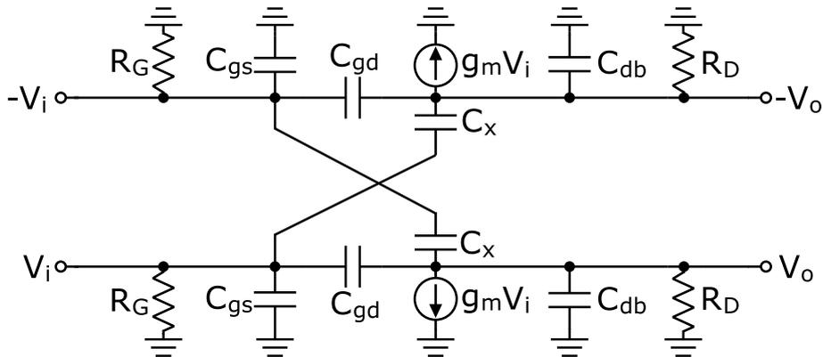
Figure 5.20: Small signal equivalent circuit of capacitive cross-coupled amplifier
