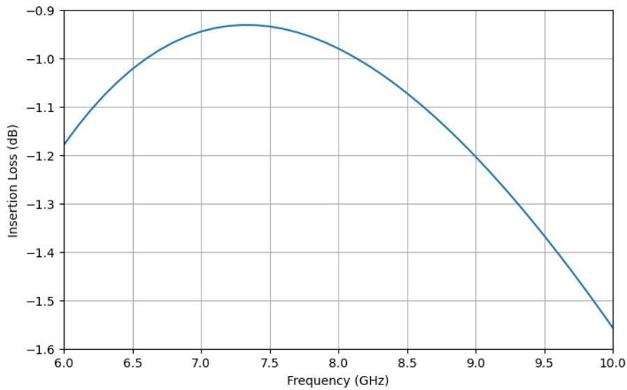
Figure 6.8: Insertion loss of the interstage balun including the matching capacitor  $C_m$
