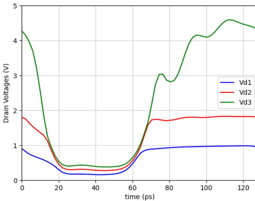
Figure 6.9: Drain voltages without the RC network
