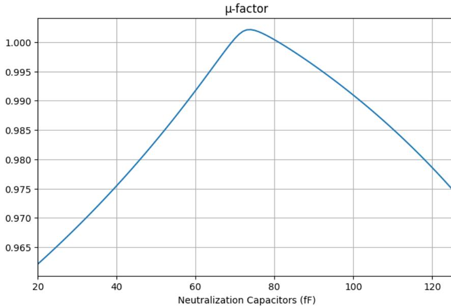
Figure 6.3:  $\mu$ -factor versus  $C_x$ .
