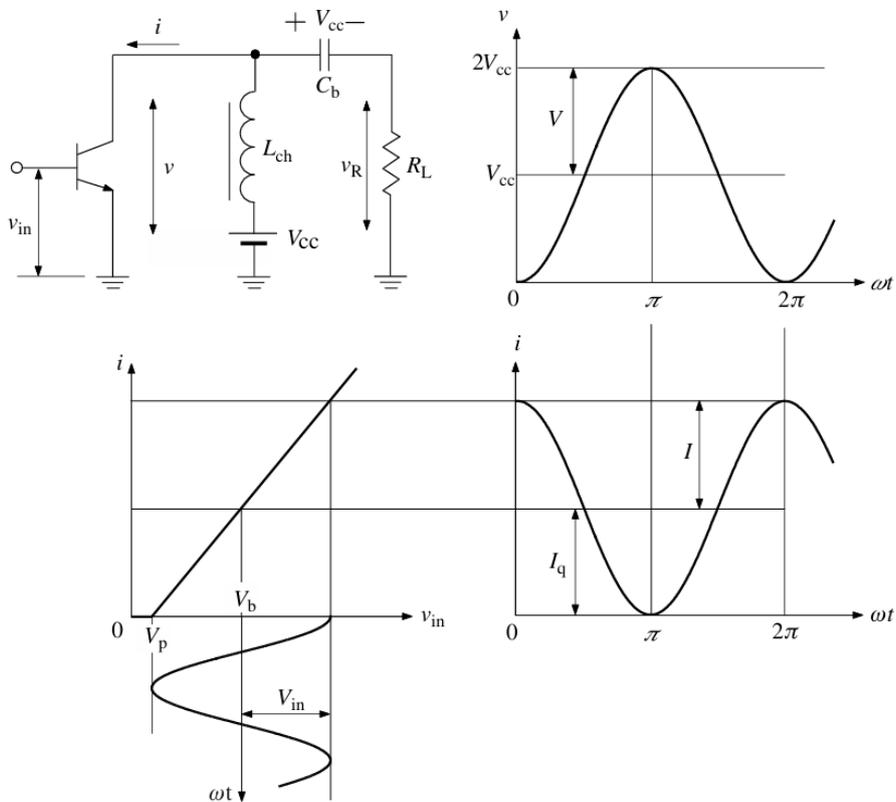
Figure 5.4: Voltage and current waveforms in Class A operation [3]
