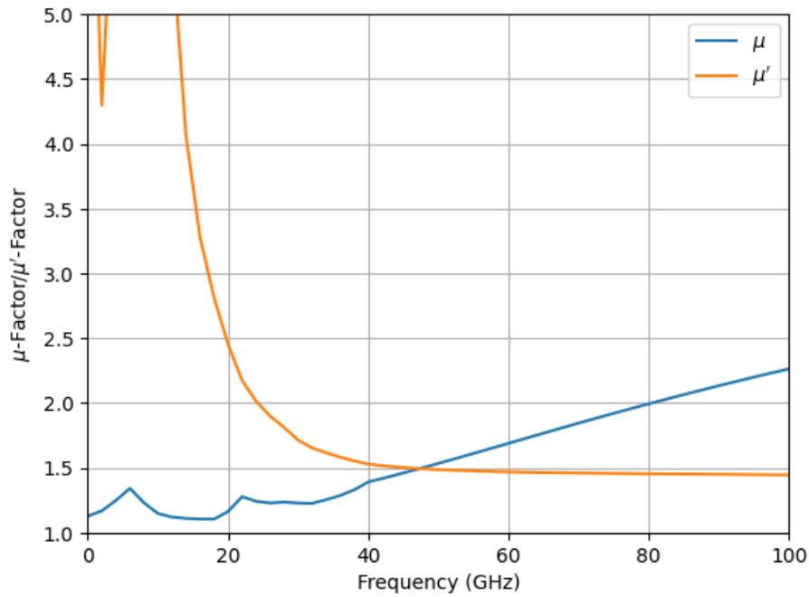
Figure 6.23: Post-layout stability factors  $\mu$  and  $\mu'$  of the power amplifier stage
