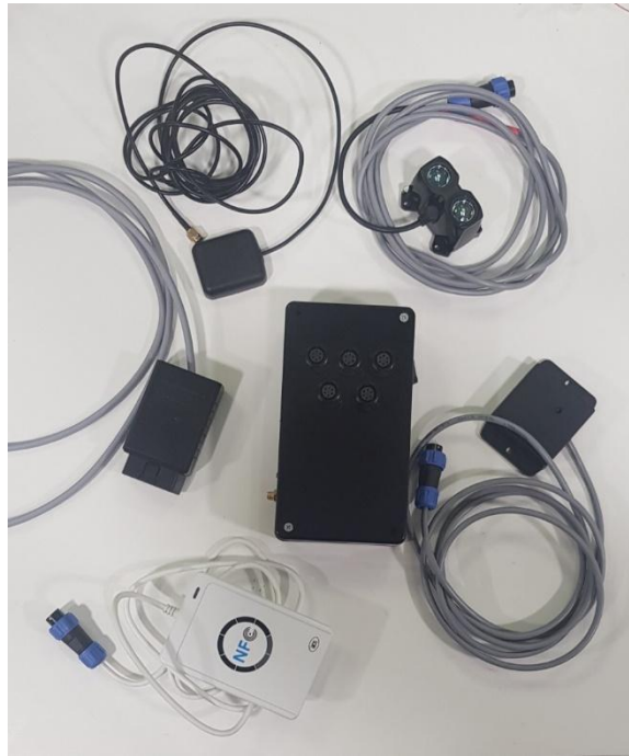
Figure 33: WINGS OBU (with integrated 5G chipset) & connected on-board sensors
