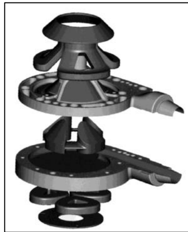
Figure 40. An exploded assembly view of the pump shows the yokes (outermost), coils, housing, and impeller.
