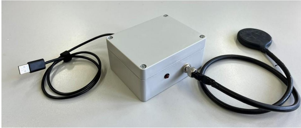
Figure 5: The final device, consisting of the waterproof sensor and the electronics enclosure.
