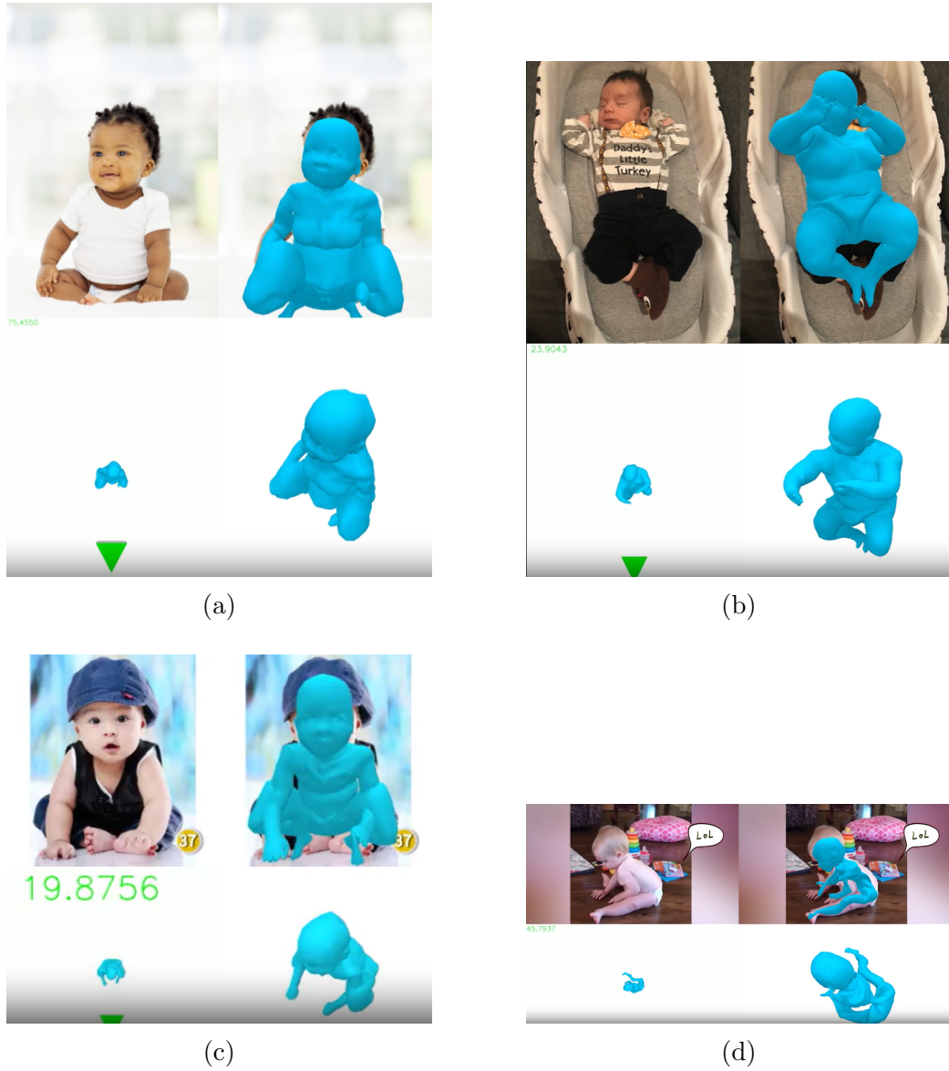
Figure 7.10: Visualizing the optimization method’s limitations on infant data. Challenging input conditions, including severe physical occlusions and complex poses, frequently result in anatomically implausible 3D body shape estimations.
