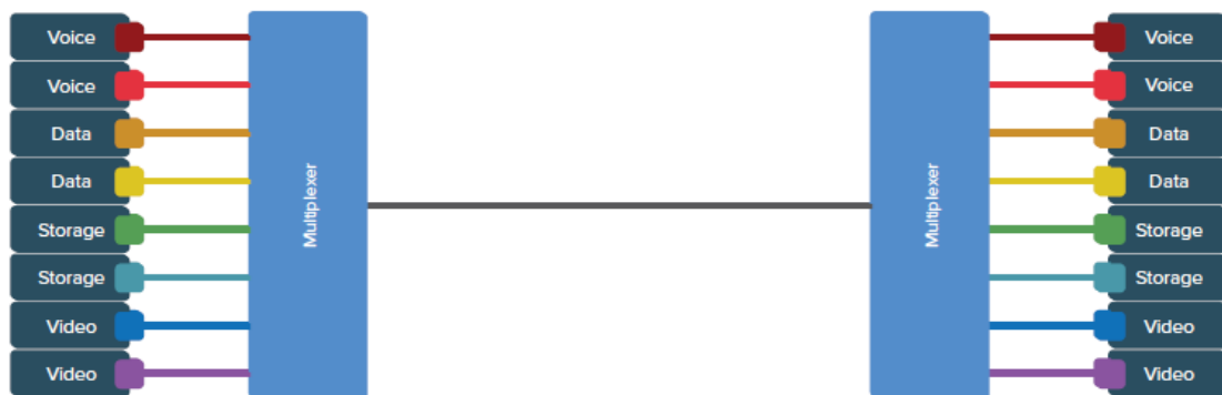
Multiplexing combines multiple channels on a single dark fiber
