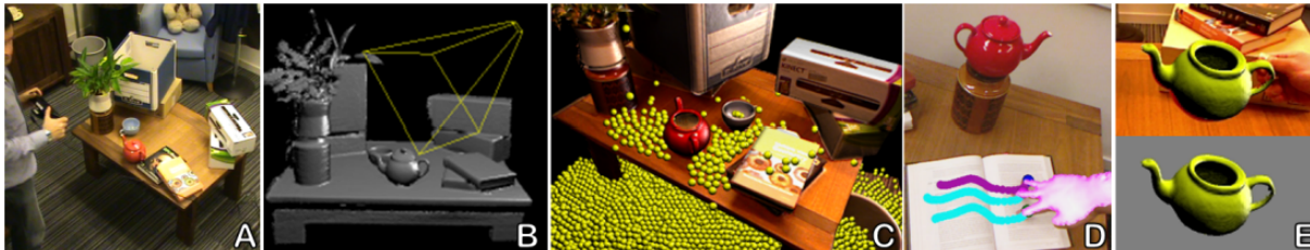
Figure 3.5.2: Demonstration of KinectFusion for real-time 3D reconstruction and interaction using a Kinect depth camera. (A) User scanning an indoor scene with Kinect. (B) Phong-shaded 3D reconstruction with wireframe frustum showing the tracked pose. (C) Texture-mapped 3D model reconstructed from Kinect RGB-D data. (D) Multi-touch interaction on the reconstructed surface. (E) Real-time segmentation and tracking of a physical object. [47]
