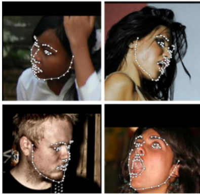
Figure 3.3.1: Facial landmark topology extracted by the Face Alignment Network [8].
