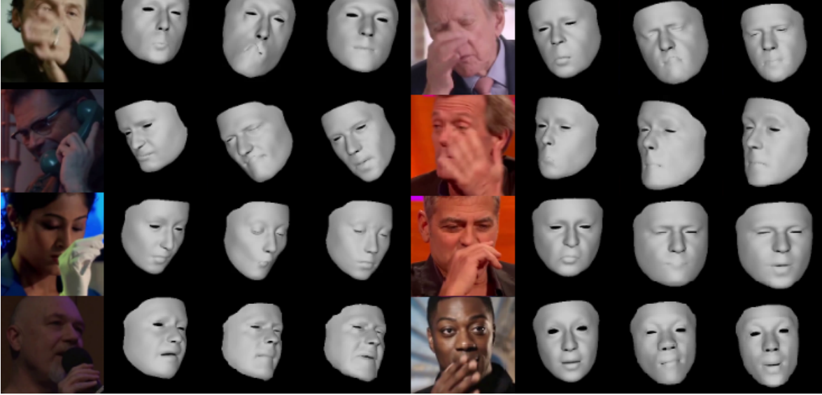
Figure 6.2.3: Visual comparison of 3D face reconstruction on unseen data for selected frames of video sequences. From left to right: Input, SPECTRE, SMIRK, ours.
