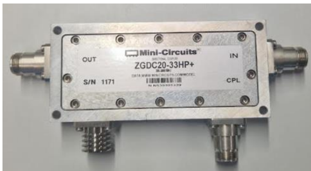
Figure 6.20: Picture of a High-Power Directional Coupler and an Attenuator
