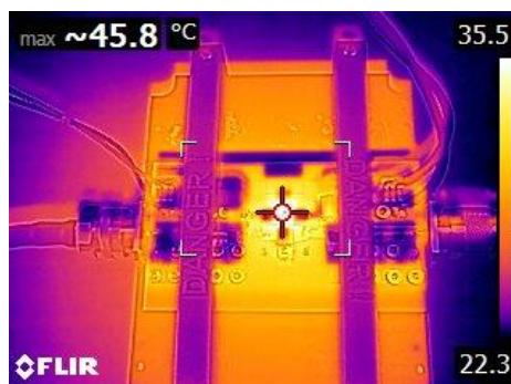
Figure 6.34: Picture from thermal camera monitoring transistor temperature of soldered transistor in pulsed mode
