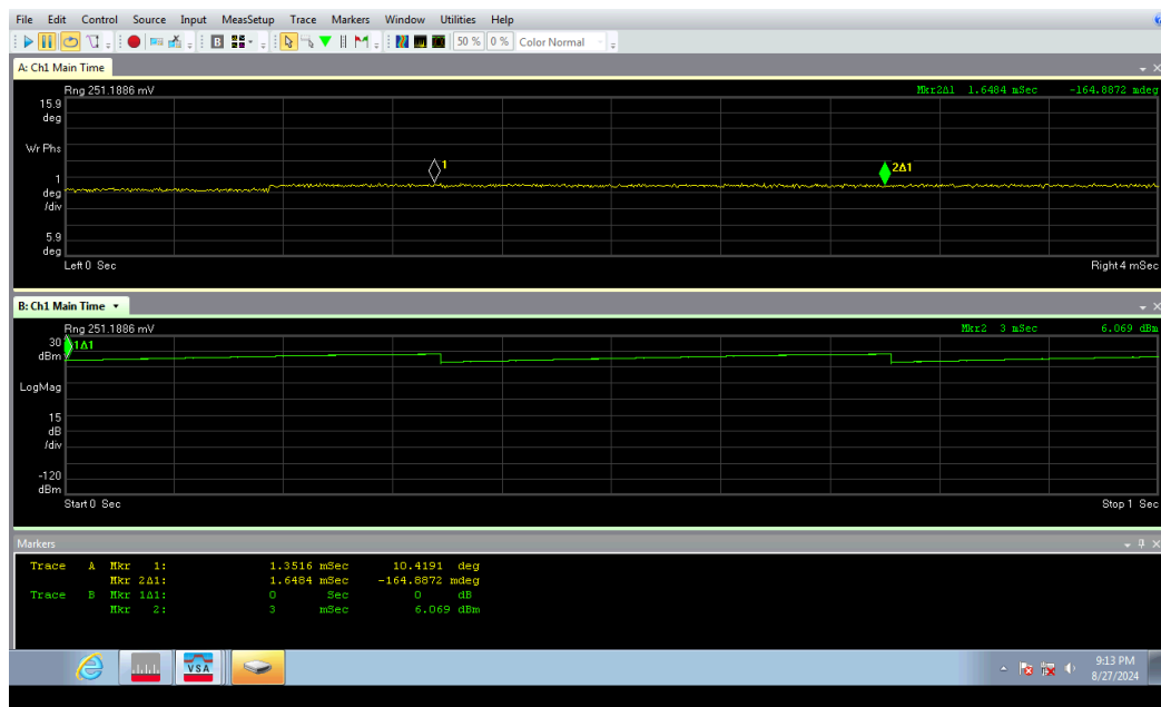
Figure 6.39: Signal Analyzer measurements for phase stability over 10dB dynamic (b)
