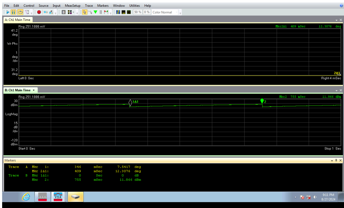
Figure 6. 38: Signal Analyzer measurements for phase stability over 10dB dynamic (a)
