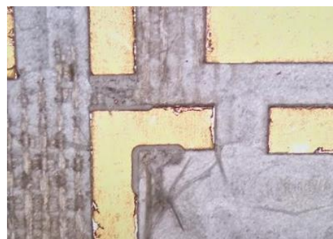
Input coupling capacitor and choke resistor
