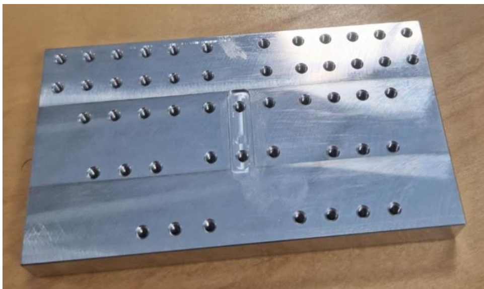
Figure 5.30: Picture of heatsink
